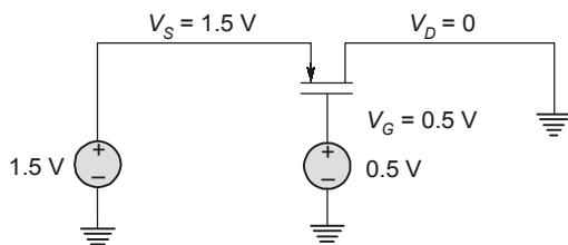
$V_{SD} > V_{SG} + V_{TH} \rightarrow$  current saturation
