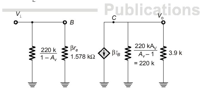
$$V_o = -(220\text{ k} \parallel 3.9\text{ k}) \beta I_B$$
