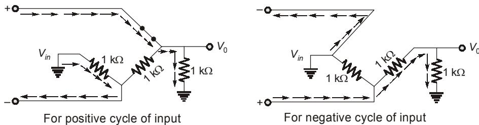
Thus the  $V_{in}$  will appear across the series combination of the two  $1\text{ k}\Omega$  resistors and we are taking output across  $1\text{ k}\Omega$  resistance only hence the output will be reduced by 50 % and the above circuit will work as a full wave rectifier with an attenuation of  $1/2$ .
